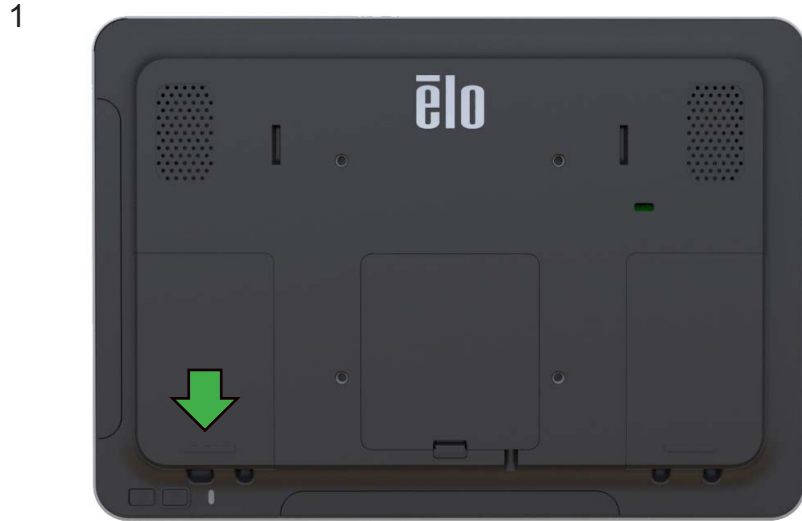
Remove the left side cable cover by sliding downward
