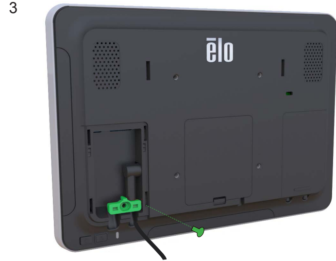
Secure the power cable using the included cable clamp and screw and replace the cable cover. The system must be connected to a network for software setup. Connect an ethernet cable now or setup wifi in step 5.
